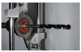
Picture showing Mortise Jig fitted with Morris MTA10 and a Morris ET101200 HSS drill bit
